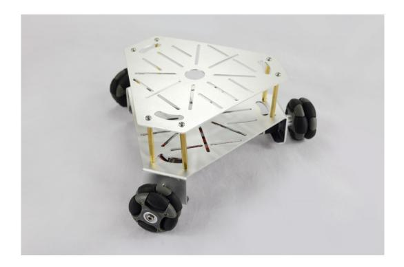
This chassis is made using robust aluminum alloy for a reliable performance. It comes with encoder embedded DC motors, and pre-drilled screw holes for easy extension.
