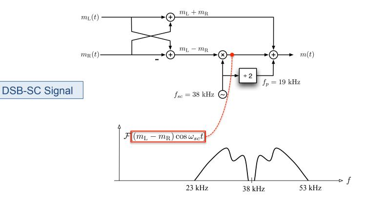
**DSB-SC signal:**  $(m_L - m_R) \cos \omega_{sc} t$  with carrier frequency  $f_{sc} = 38 \text{ kHz}$ .
