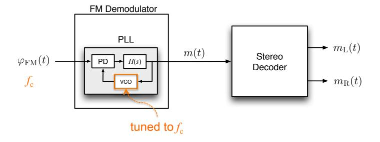
• Use a PLL with its VCO tuned to the carrier frequency  $f_c$  of the incoming FM signal to demodulate and generate the baseband signal m(t).
