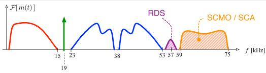
$$m(t) = [m_L + m_R] + [m_L - m_R] \cos \omega_{sc}t + K_p \cos \omega_p t + K_r \varphi_r(t) + K_s \varphi_s(t)$$
