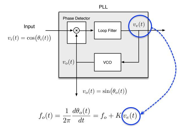
PLL is a feedback control system such where the output of the loop filter controls the instantaneous frequency of the VCO:
