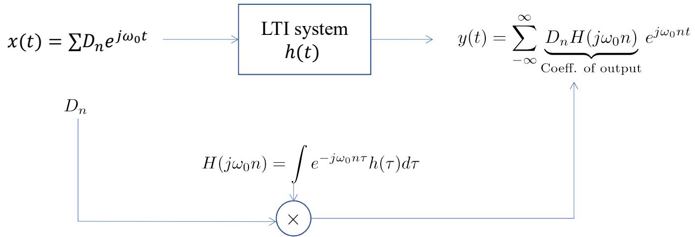
It is faster to find the Convolution results using  $H(j\omega_0 n)$ s and Fourier Series Coefficients
