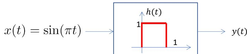
To Find output of an LTI system to a periodic input  $x(t)$ :
