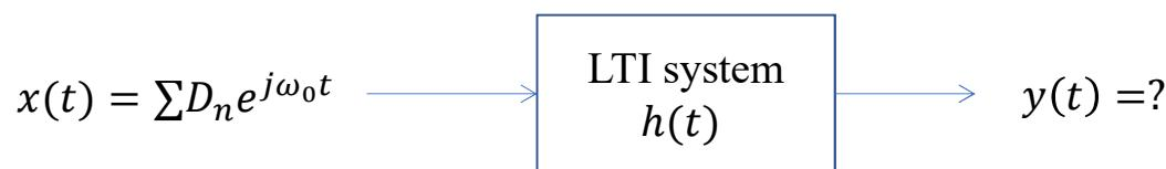
$$\begin{aligned} y(t) &= x(t) * h(t) \\ &= \left( \sum_{-\infty}^{\infty} D_n e^{j\omega_0 n t} \right) * h(t) \\ &= \sum_{-\infty}^{\infty} D_n (e^{j\omega_0 n t} * h(t)) \\ &= \sum_{-\infty}^{\infty} \underbrace{D_n H(j\omega_0 n)}_{\text{Coeff. of output}} e^{j\omega_0 n t} \end{aligned}$$
