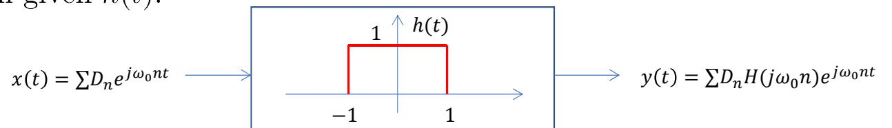
To Find output of an LTI system to a periodic input  $x(t)$ :
