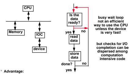
• Simple: the processor is totally in control and does all the work
