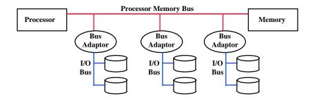
$^\circ\,$  I/O buses tap into the processor-memory bus via bus adaptors:
