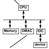
CPU sends a starting address, direction, and length count to DMAC. Then issues "start".
