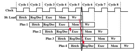
° In the Simple Pipeline Processor if a Load is fetched during Cycle 1:
