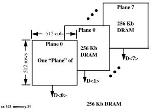
Logic Diagram of a Typical DRAM
