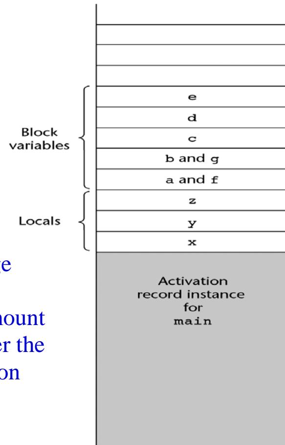
2. Since the maximum storage required for a block can be statically determined, this amount of space can be allocated after the local variables in the activation record
