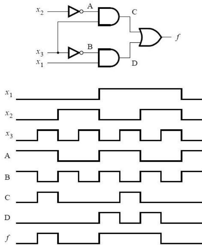
2.9. Timing diagram of the waveforms that can be observed on all wires of the circuit:
