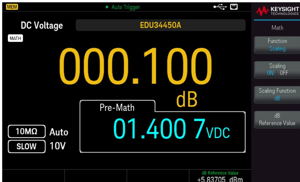
The reading before the math formula is applied is shown in the secondary display.
