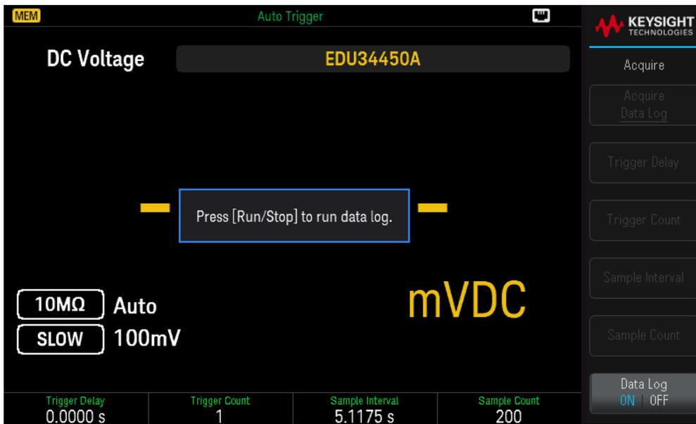
Press **[Run/Stop]**. Data logging will begin immediately or following the specified Trigger Delay (if Trigger Count is > 1).
