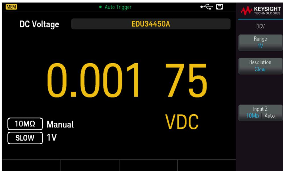
3. Press [Shift] > [Display] > 2nd Meas ON | OFF to enable the secondary measurement.
