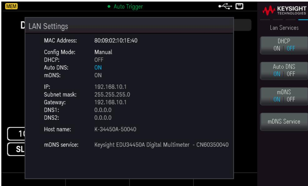
Press **[Back]** > **Addresses** > **Modify** to configure the IP address, subnet mask, and gateway address.
