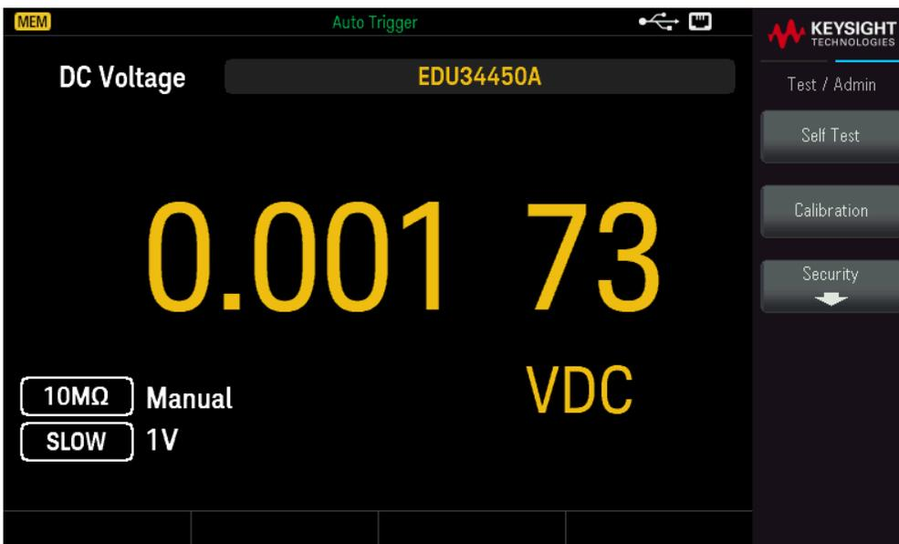
**Self Test** verifies proper instrument operation. This self-test is equivalent to the \*TST? SCPI query, and you do not need to remove inputs to the instrument to run the test.
