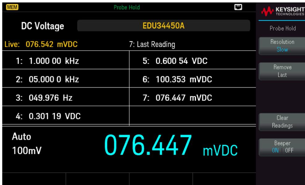
The captured reading is shown on the bottom of the display. The live reading is shown at the top left of the display.
