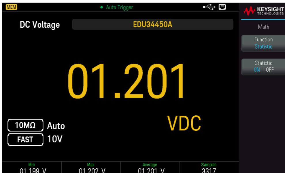
The minimum, maximum, and average readings together with the number of samples taken are shown on the bottom of the display.
