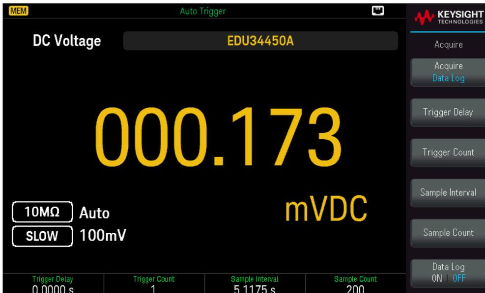
You can then select the sample interval (time between measurements - for example, 500 ms), duration as either an amount of time or a number of readings, and whether to start after a delay.
