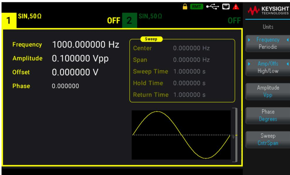
2. Press [Sweep] > **Center** or **Span**. Use the numeric keypad or the knob and arrows to set a desired value. If you use the keypad, select a prefix unit to finish.
