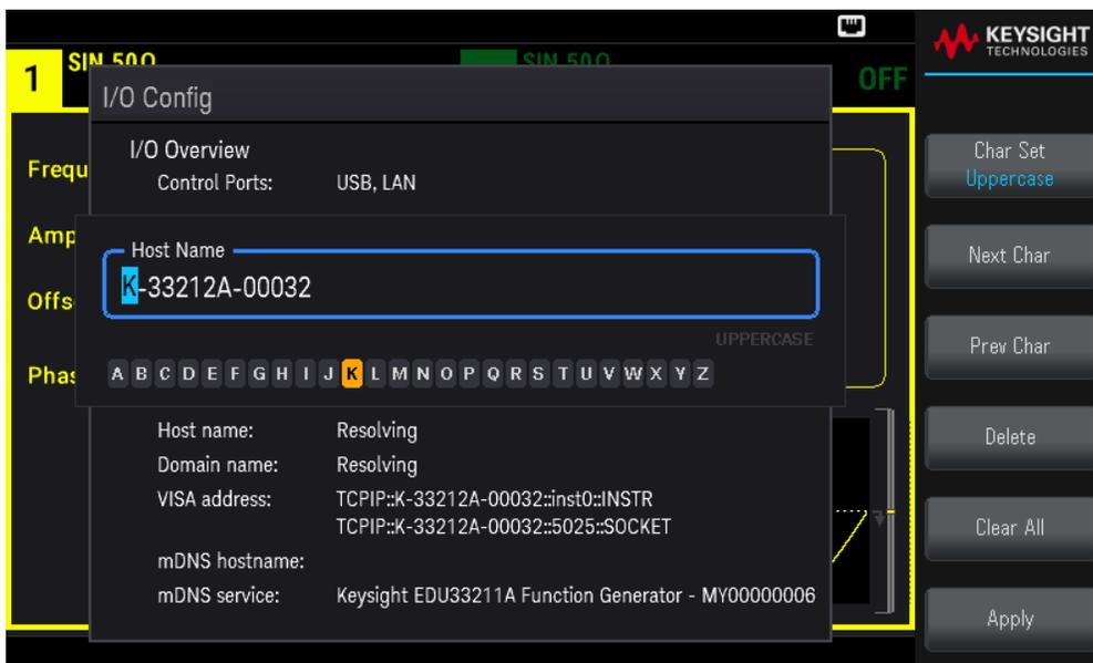
The instrument is shipped with a default hostname with the following format: K-{modelnumber}-{serialnumber},
