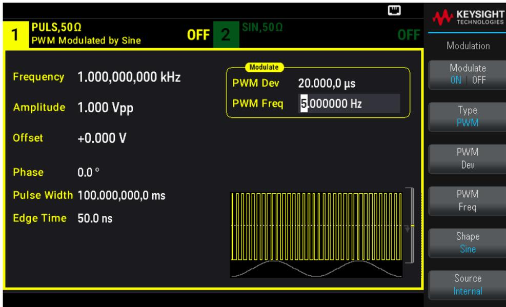
To view the actual PWM waveform, you would need to output it to an oscilloscope. If you do this, you will see how the pulse width varies, in this case, from 80 to 120  $\mu$ s. At a modulation frequency of 5 Hz, the deviation is easily visible.
