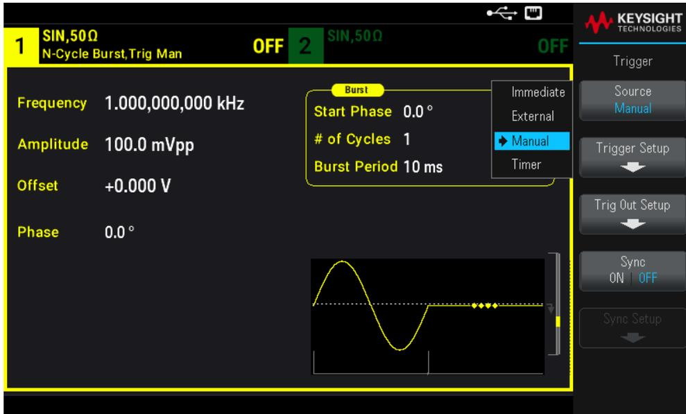
If sweep or burst is on, pressing **[Trigger]** displays the trigger menu. An illuminated **[Trigger]** key (solid or blinking) indicates that one or both channels are awaiting a manual trigger. Solid illumination occurs when the trigger menu is selected, and flashing illumination occurs when the trigger menu is not selected. The **[Trigger]** key is disabled when the instrument is in remote.
