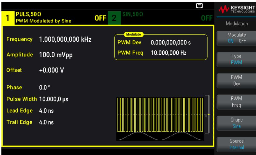
The waveform is output using the present carrier and modulating waveform settings.
