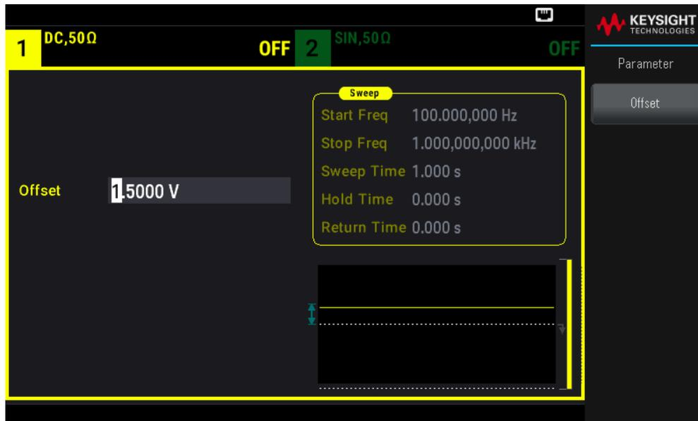
2. Enter the desired voltage offset. Enter 1.0 with the numeric keypad or knob, and press the V softkey if you used the keypad.
