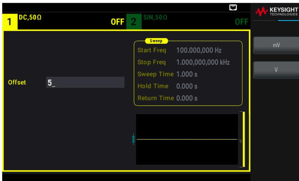
2. Press Channel [On/Off] to produce the DC output.
