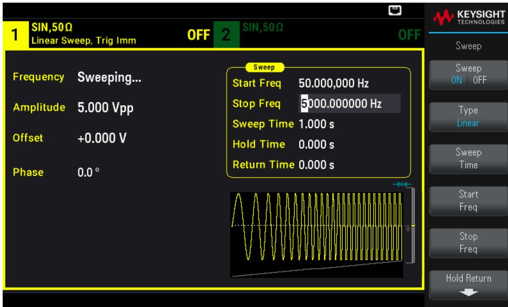
At this point, the instrument outputs a continuous sweep from 50 Hz to 5 kHz if output is enabled.
