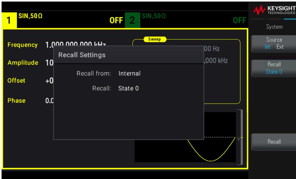
If choose to recall an instrument state file from the instrument's non-volatile internal memory, select **Int**. Proceed to step 2.
