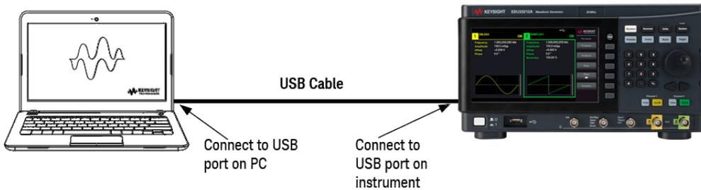
1. Connect your instrument to the USB port on your computer using a USB cable.
