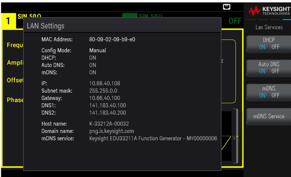
With DHCP on, an IP address will automatically be set by the DHCP (Dynamic Host Configuration Protocol) when you connect the instrument to the network, provided the DHCP server is found and is able to do so. DHCP also automatically deals with the subnet mask and gateway address, if required. This is typically the easiest way to establish LAN communication for your instrument. All you need to do is leave DHCP on. Contact your LAN administrator for details.
