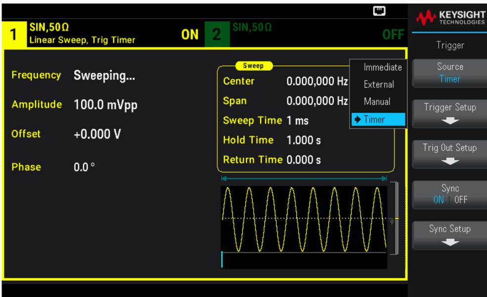
To specify the slope of the trigger signal edge: Press [Trigger] > Trig Out Setup > Trig Out **Off** | (Up) | (Down).
