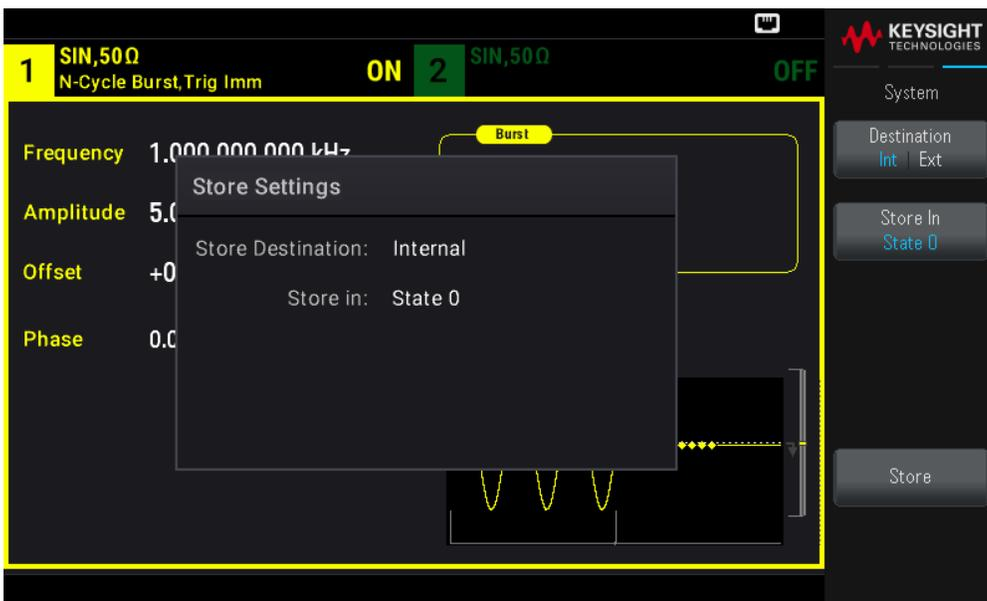
If choose to store the instrument state in the instrument's non-volatile internal memory, select **Int**. Proceed to step 2.
