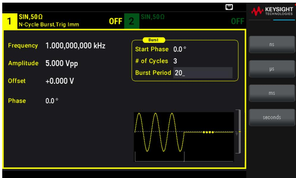
You can generate a single burst (with the specified count) by pressing the **[Trigger]** key. For more information, see [Trigger a Sweep or Burst](#).
