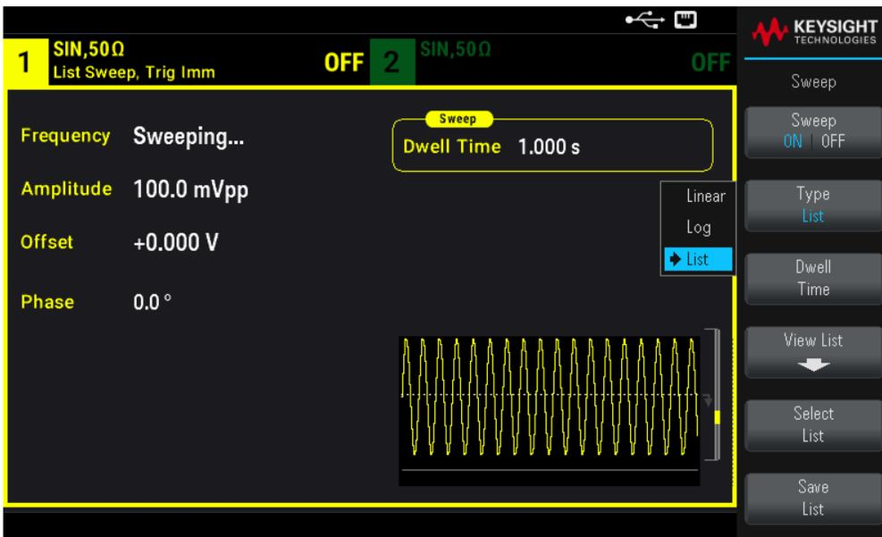
Select **View List** to view the list parameters. You can edit (**Edit Freq**) the frequency value in the sweep list, add (**Add Freq**) or delete (**Delete Freq**) a frequency value, and reorder the sweep list (**Reorder List**).
