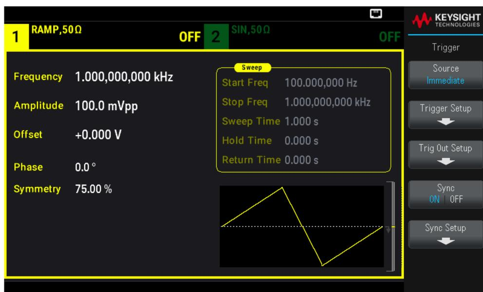
To configure Sync: Press `[Trigger]` > `Sync Setup`.
