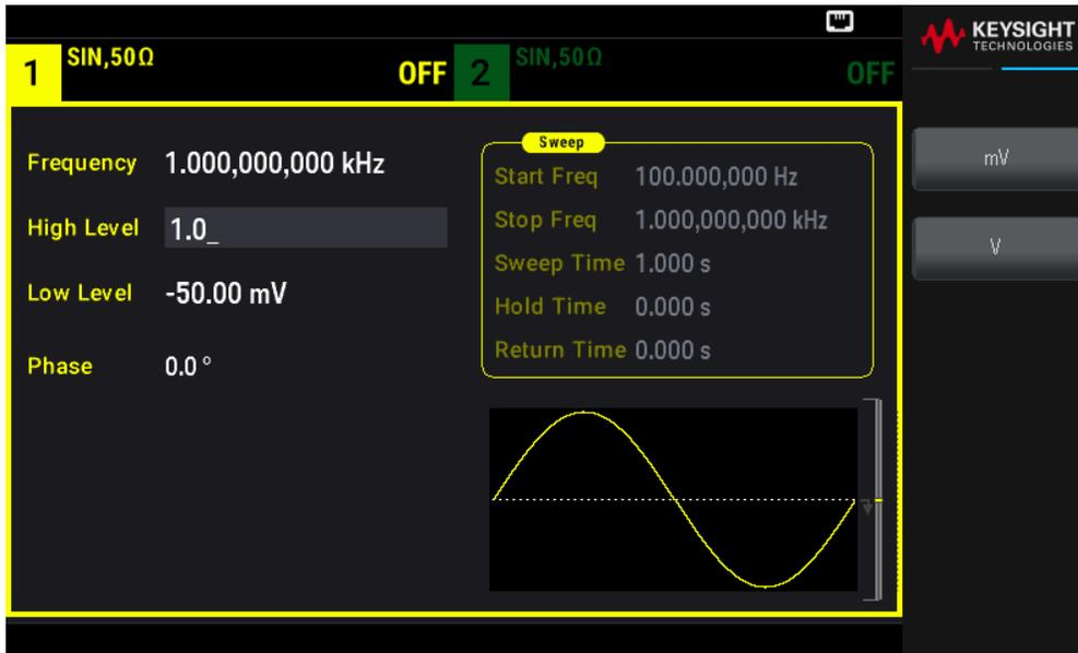
3. Press the Low Level softkey and set the value. Again, use the numeric keypad or the knob to enter a value of 0.0 V.
