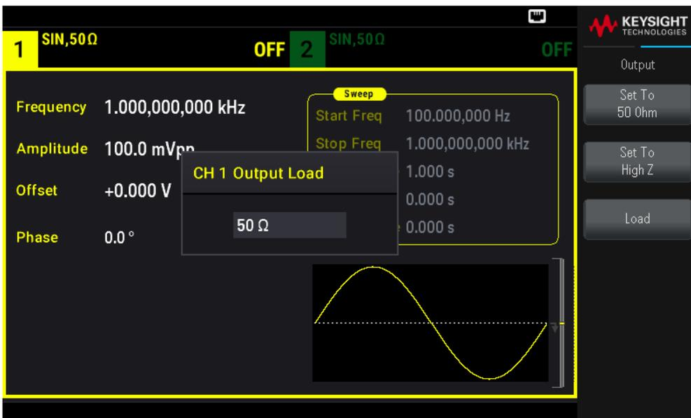
3. Select the desired output termination either by using the knob or numeric keypad to select the desired load impedance or by pressing **Set to 50 Ω** or **Set to High Z**. You can also set a specific value by pressing **Load**.
