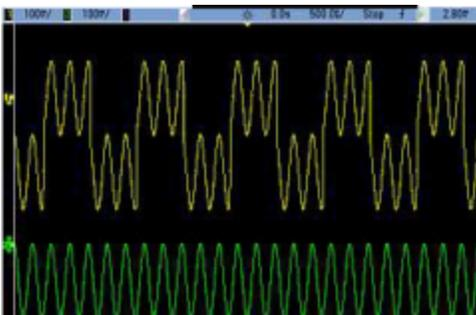
You may also use Combine with bursts. For example, consider the image below, which includes a 1 kHz sine wave on channel 1 and three-cycle bursts of a 5 kHz sine wave on channel 2.
