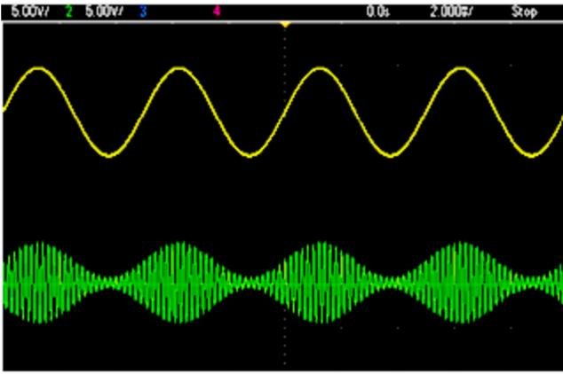
– Double-sideband suppressed-carrier (DSSC). Many modern communications systems employ DSSC on each of two carriers that have the same frequency but a 90-degree phase difference. This is called quadrature amplitude modulation (QAM).
