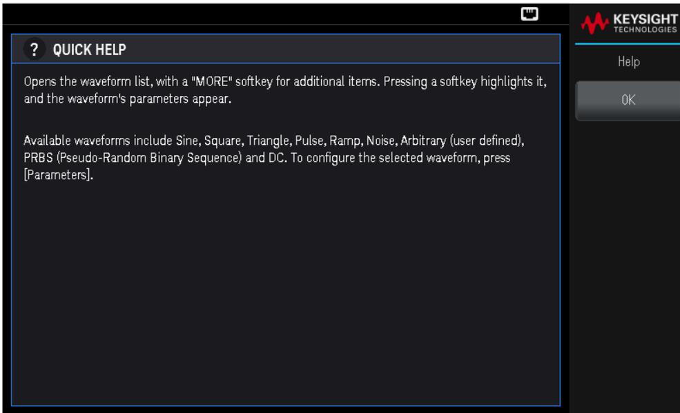
If the message contains more information than will fit on the display, press the down arrow softkey to view the remaining information.
