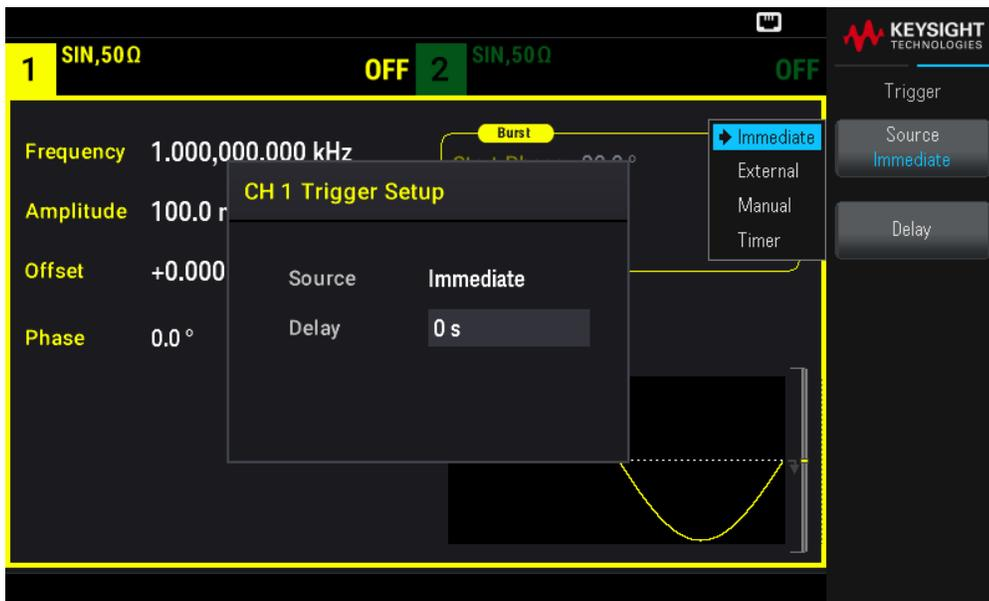
To specify whether the instrument triggers on a rising or falling edge of the signal at the **Ext Trig** connector, select the external trigger source before choosing **Trigger Setup**.
