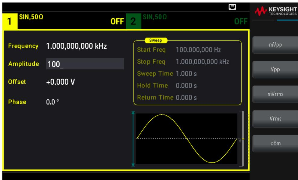
To use a high level and low level instead: Press **[Units]** > **Ampl/Offs** | **High/Low**.
