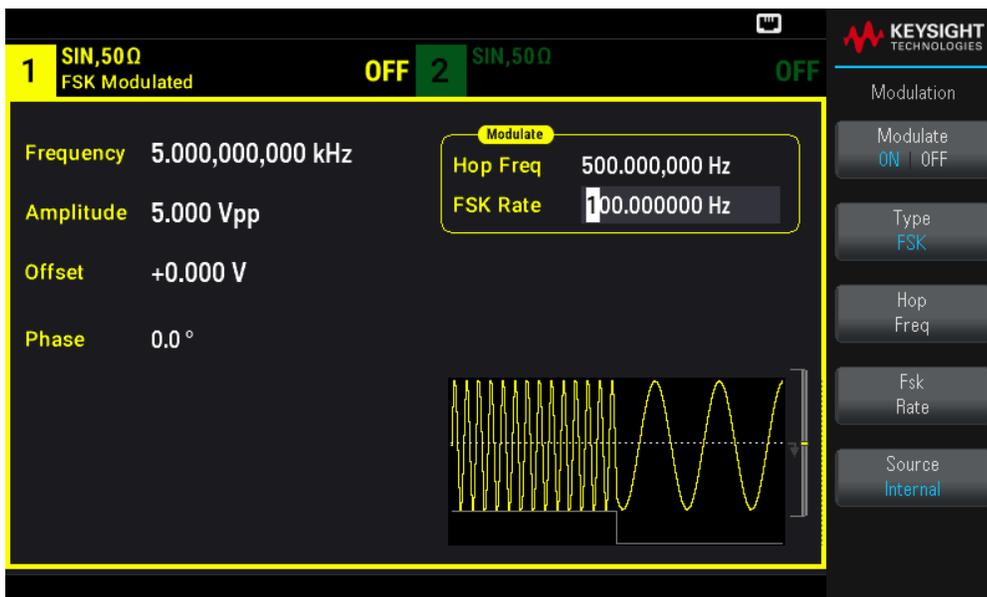
At this point, the instrument outputs an FSK waveform if the channel output is enabled.
