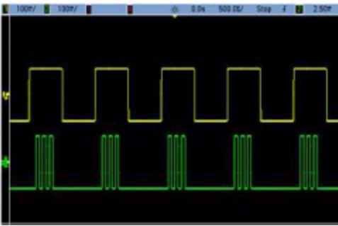
When these signals are combined on channel 1, the result is a simple amplitude addition of the two signals, as shown below.
