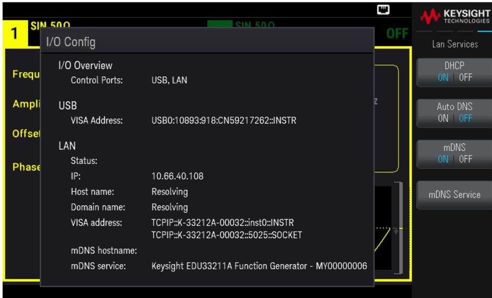
a. Set the "hostname." Press **[Back]** > **Host Name** and enter the hostname. A hostname is the host portion of the domain name, which is translated into an IP address. The hostname is entered as a string using the softkeys provided. The hostname may include letters, numbers, and dashes ("-").
