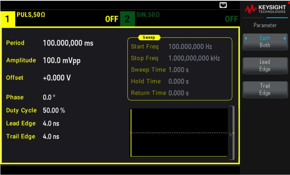
1. To set the transition times for the edges of the pulse together: Press [Waveform] > Pulse > Edge > Each **Both**.
