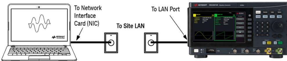
1. Connect the instrument to the site LAN or to your computer using a LAN cable. The as-shipped instrument LAN settings are configured to automatically obtain an IP address from the network using a DHCP server (DHCP is ON by default). The DHCP server will register the instrument's hostname with the dynamic DNS server. The hostname as well as the IP address can then be used to communicate with the instrument. The front panel **LAN** indicator will come on when the LAN port has been configured.
