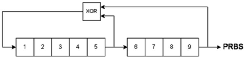
An LFSR is specified by the number of stages it contains and which stages ("taps") feed the exclusive-or (XOR) gates in its feedback network. The PRBS output is taken from the last stage. With properly chosen taps, an L-stage LFSR produces a repetitive PRBS of length  $2^L - 1$ . The clocking frequency of the LFSR determines the "bit rate" of the PRBS.
