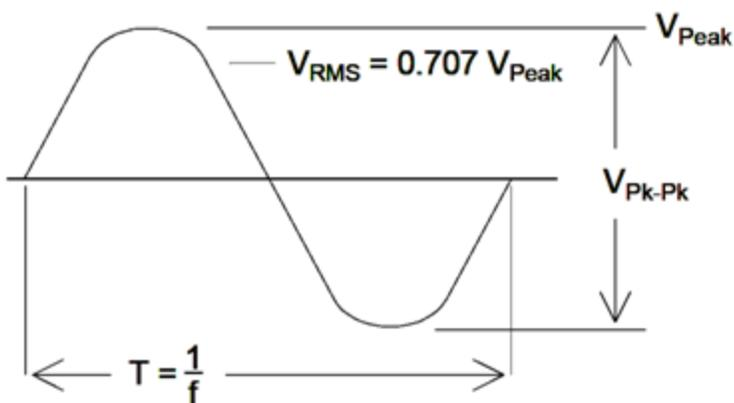
A waveform's peak voltage is the maximum absolute value of all of its points. The peak-to-peak voltage is the difference between the maximum and minimum. The RMS voltage equals the standard deviation of all waveform points; it also represents the one-cycle average power in the signal, minus the power in any DC component of the
