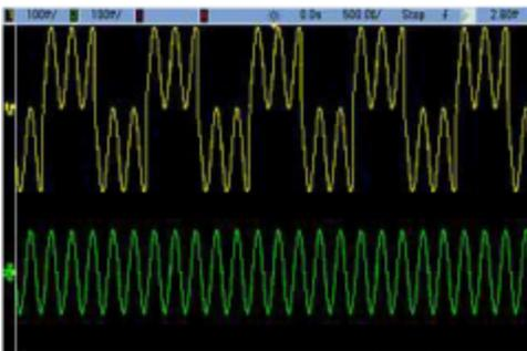
When signals are combined, the DC Offset values are not added together. Only the DC Offset from the receiving channel is used in the combined output. The figure below shows 50 a mV DC Offset added to Channel 1. The 50 mV offset added to Channel 2 is ignored.
